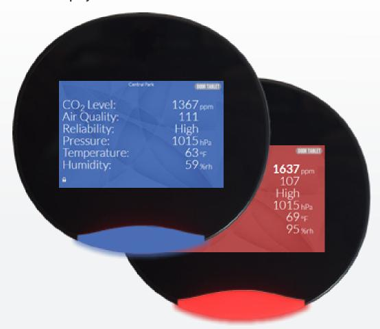
Our Sensors send a message to your devices and change the entire screen to red when the established threshold is passed, in order to immediately alert staff.
